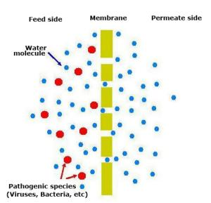
(including *Escherichia coli*, *Salmonella typhi* and *Vibrio cholera*). The modules filter solutes of molecular weight more than 60,000 dalton. However, it does not remove dissolved salts of small particle size.
